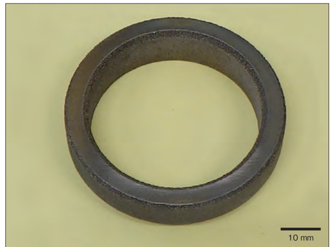
図 13 SLM で造形した Fe-Cr-Co 磁石部品の外観 Fig. 13 Appearance of an additively manufactured Fe-Cr-Co magnet part
