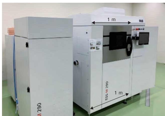
図2 EOS M290の外観 Fig.2 Appearance of EOS M290
