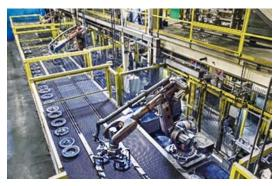
Fig. 2 Dual-station core machine with robot cell
