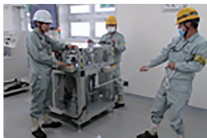
Learning system that simulates being caught by rotating equipment This system provides a firsthand experience of what it is like if fabric or strings are wrapped up in the rotating axis of machinery. Even a motor equivalent to that of a household electric fan can generate powerful pulling force when slowed down.
