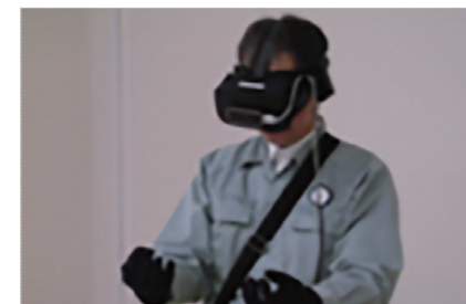
Virtual reality (VR) device The device enables users to experience the hazards of various tasks virtually. Simulating occupational accidents helps increase employees’ sensitivity to danger, leaving them with strong memories of their experiences.
