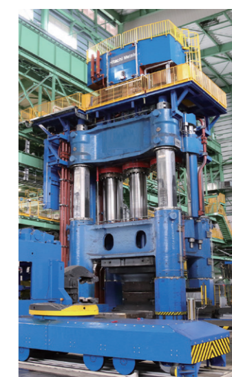
10,000 ton-class free forging press
