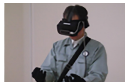
Virtual reality (VR) device The device enables users to experience the hazards of various tasks virtually. Simulating occupational accidents helps increase employees’ sensitivity to danger, leaving them with strong memories of their experiences.
