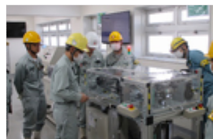
Learning system that simulates being caught by rotating equipment This system provides a firsthand experience of what it is like if fabric or strings are wrapped up in the rotating axis of machinery. Even a motor equivalent to a household electric fan can generate powerful pulling force when slowed down.
