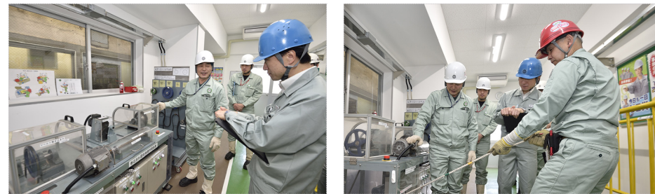
Learning system that simulates being caught by rotating equipment This system provides a firsthand experience of what it is like if fabric or strings are wrapped up in the rotating axis of machinery. Even a motor equivalent to a household electric fan can generate powerful pulling force when slowed down.
