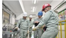
**Learning system that simulates being caught by rotating equipment**This system provides a firsthand experience of what it is like if fabric or strings are wrapped up in the rotating axis of machinery. Even a motor equivalent to a household electric fan car generate powerful pulling force when slowed down
