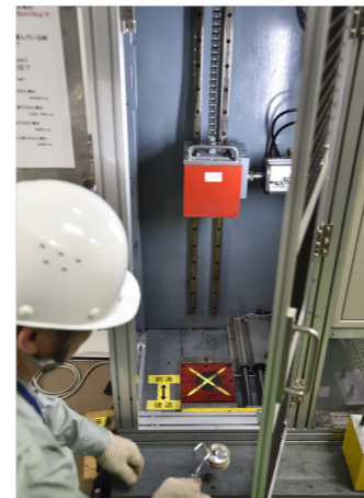
Learning system that simulates the impact force from falling objects This system demonstrates how a 25-kilogram weight dropped from a height of one meter generates enough impact force to crush an empty drink can. This increases safety awareness when transporting steel ingots.
