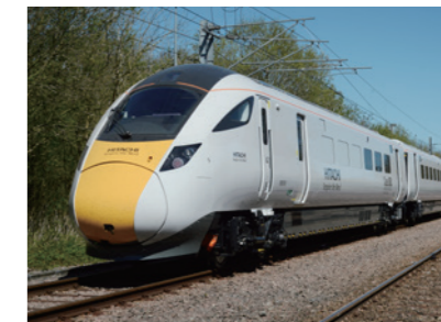
Class 800 train manufactured for the Intercity Express Programme (IEP) in the United Kingdom (order received by the Hitachi Group)
