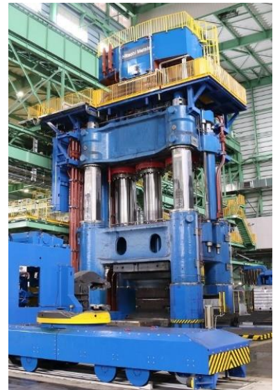
10,000-ton free forging press
