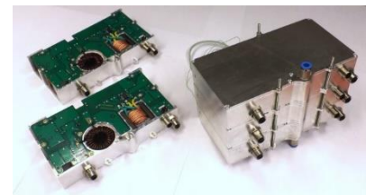
OBC prototypes Single-phase kilowatts: 3.6 (left) Three-phase kilowatts: 11 (right)
