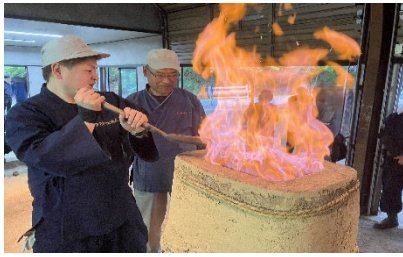
Insertion of iron sand and charcoal Destruction of furnace and removal of kera Kera (including tamahagane) Photos from a past replication of the ancient Tatara steelmaking method
