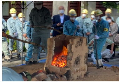
Insertion of iron sand and charcoal Destruction of furnace and removal of kera Kera (including tamahagane) Photos from a past replication of the ancient Tatara steelmaking method
