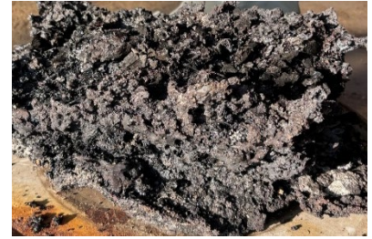
Insertion of iron sand and charcoal Destruction of furnace and removal of kera Kera (including tamahagane) Photos from a past replication of the ancient Tatara steelmaking method
