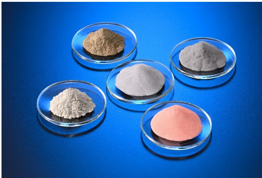
Photograph 2. Plated Ni-P particles Center: no plating. Left: silver plating. Top: gold plating. Bottom: copper plating. Right: solder plating.
