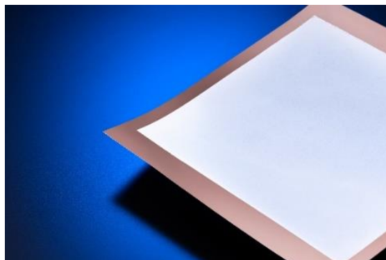
Appearances of samples made by applying ALectro (The white part is the electrodeposited aluminum) (Left: A metal block whose entire surface is coated by applying ALectro, Right: A copper foil coated by applying ALectro)
