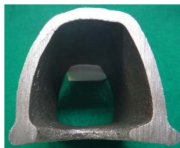
Cross-sectional photograph of the hollow opening of the OMEGA KNUCKLE®
