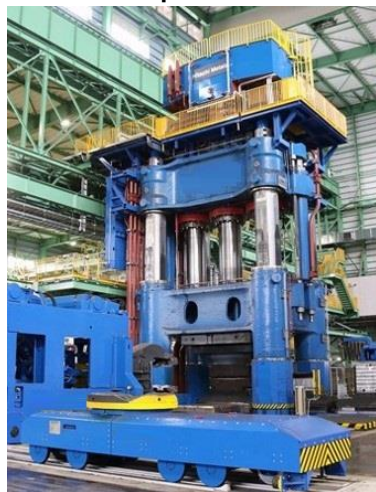
10,000-ton forging press
