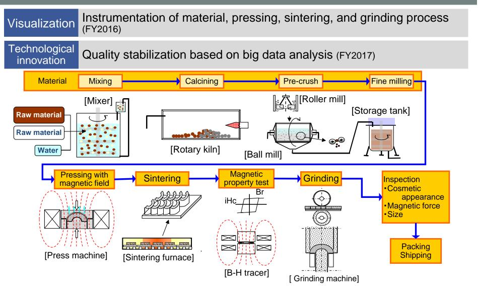
Establish innovative production line at Kumagaya Works (Operation in FY2018)  $\Rightarrow$  Global rolling out of achievements
